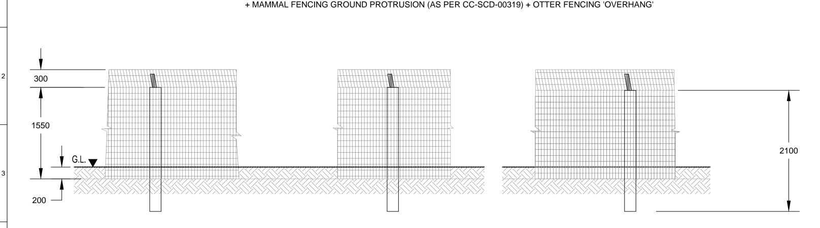
TIMBER POST AND TENSIONED WIRE MESH FENCING (AS PER CC-SCD-00320)
